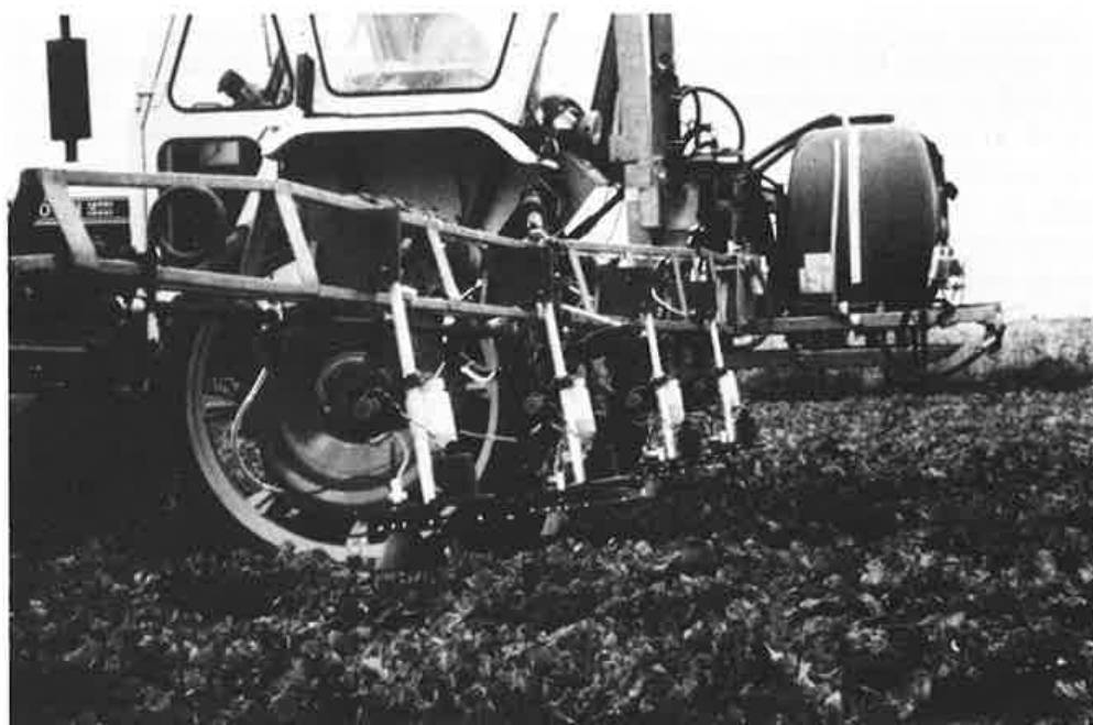
Tractor-mounted electrostatically-charged rotary atomizers are improving spraying efficiency and preventing drift
