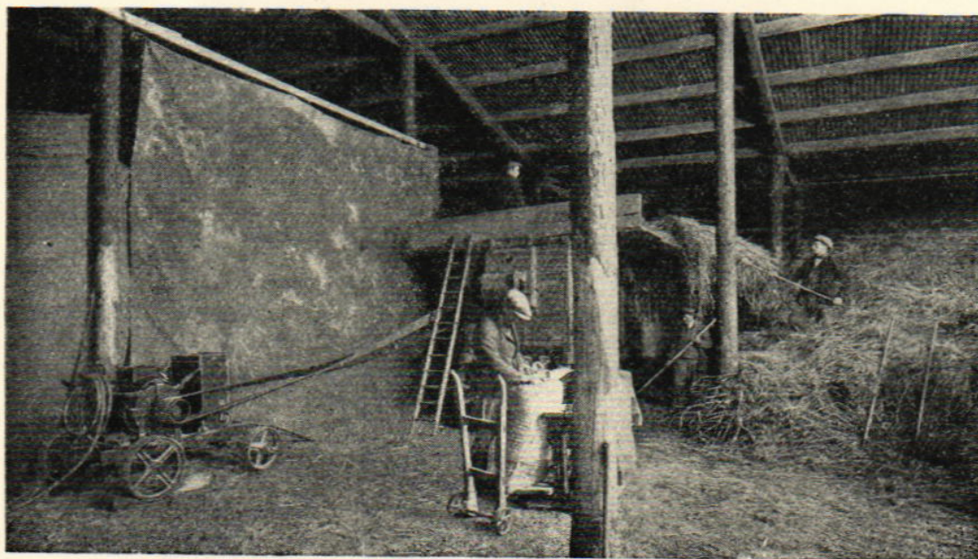
Fig. 11. 20 h.p. heavy duty portable motor driving thresher.
